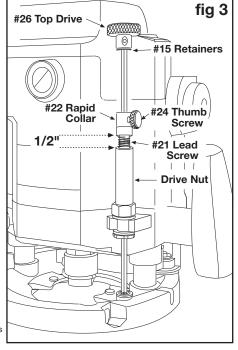
**Router Raizer Parts Required:** (see page 1) #1, #2, #4, #7, #11, #12, #13, #14, (three #15) #16, #18, #19, #21, #22, #23, #24, #25, #26, #27, #28, #29, (#30, #31, #46 for router table installation).
